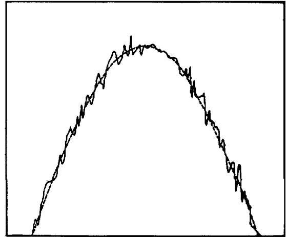
Figure 2-7. SIGNAL VOLTAGE WITH CONVERTER NOISE
